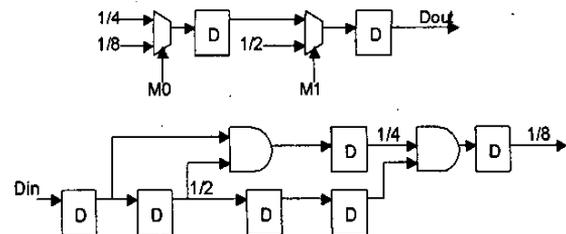
Figure 4. Schematic of the mark density generator. Its inputs are the two select signals  $M_0$ ,  $M_1$  and the output of the core. Its output is the pattern output, which also goes into the Error detector circuit.
