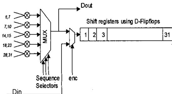
Figure 3. High-level diagram of the PRBS core. The numbers shown are the taps from the shift register. Its inputs are the three sequence selectors ( $s_0$ ,  $s_1$ ,  $s_2$ ), the input stream  $D_{in}$  (needed only in detector mode) and the clock. Its output is the  $D_{out}$ .
